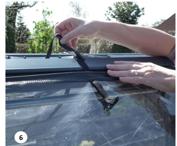
6) Close the side overnight and attach any bindings from the opposite side.
